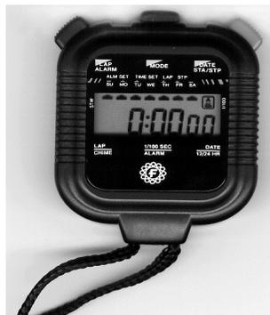
The stopwatch will be used to measure the time it takes to complete a task from the beginning of the activity until the conclusion. Press the middle (mode) button to make sure you are in stopwatch mode. The display should read **0:0000**. To time the task, just press the right-hand button (labeled STA/STP) at the top of the stopwatch to begin, and
